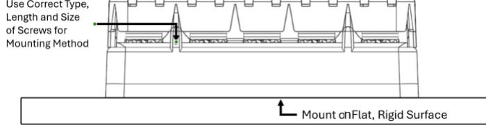
(2) Use the appropriate screw type (machine/thread cutting), size (match with pilot or through-hole diameter), and length; ensuring that the weight of the product and associate cables will be properly secured.
